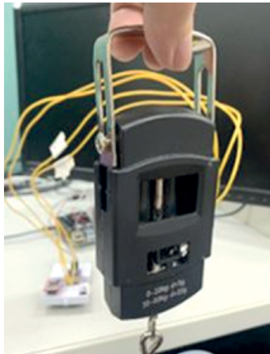
Figure 8. Urine weight sensor
